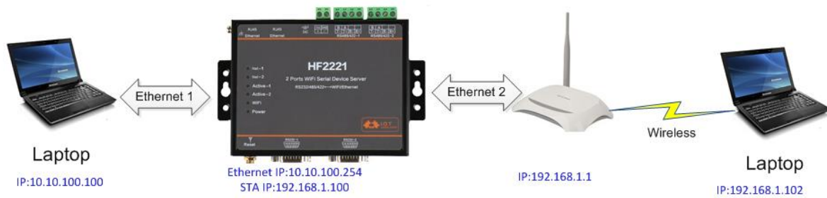
Figure 24. Ethernet Port Function2 (Bridge)
