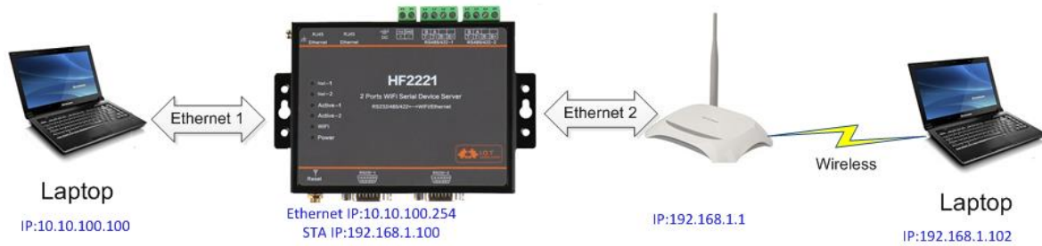
Figure 22. Ethernet Interface Function 1 (Router)
