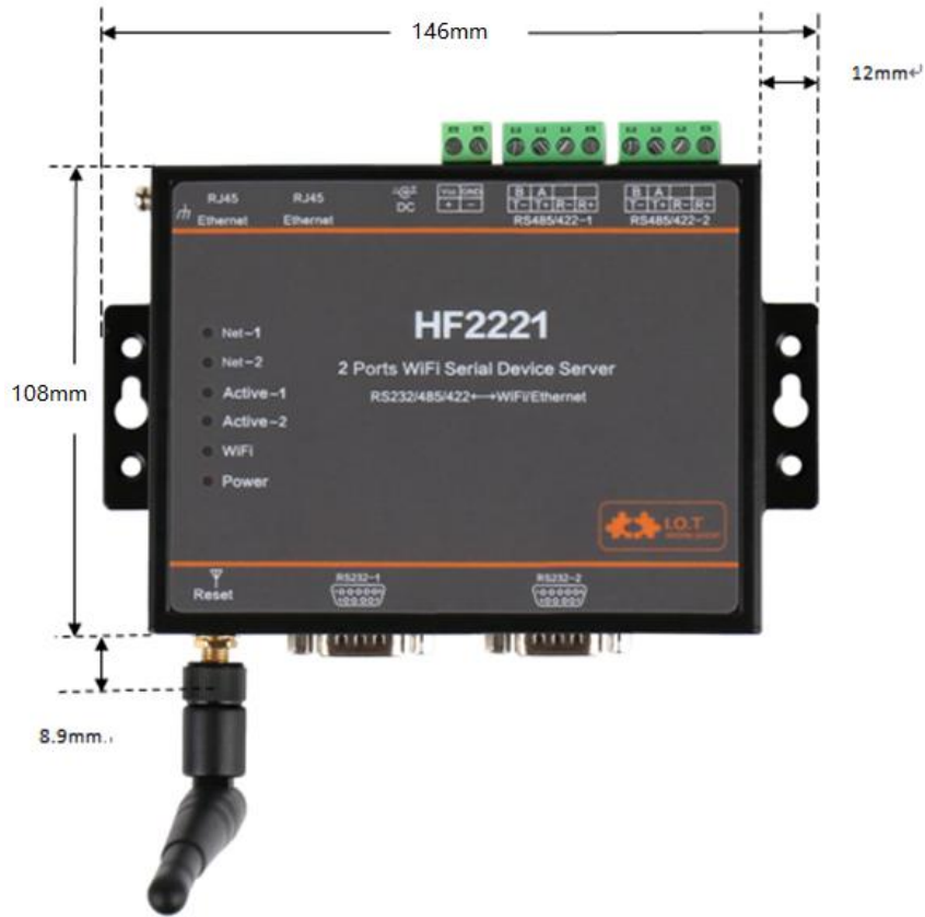
Figure 7. HF2221 Mechanical Dimension
